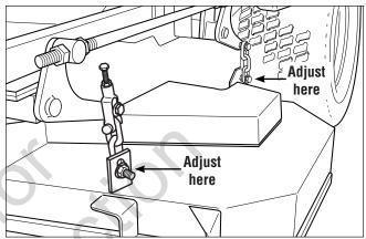
Figure 44. Hanger Chain Adjustment
